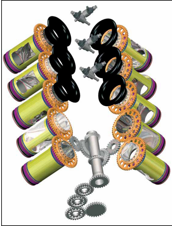
Figure 3 - Rotary valvetrain and inlet tract arrangement on a V10 F1 engine tested on dyno
